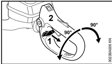
The rear handle can be turned through 90° to the left or right for better control and comfort in all cutting situations.
