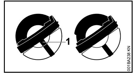
Left: Bottom of cap is twisted – inner mark (1) in line with outer mark.
