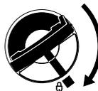
Insert the fuel cap with hinged grip (bayonet-type cap) correctly in the opening, turn it clockwise as far as stop and fold the grip down.
