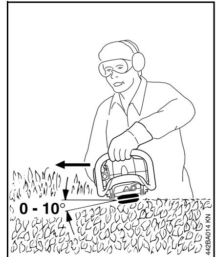
Hold the cutter bar at an angle of  $0^\circ$  to  $10^\circ$  as you swing the hedge trimmer horizontally.
